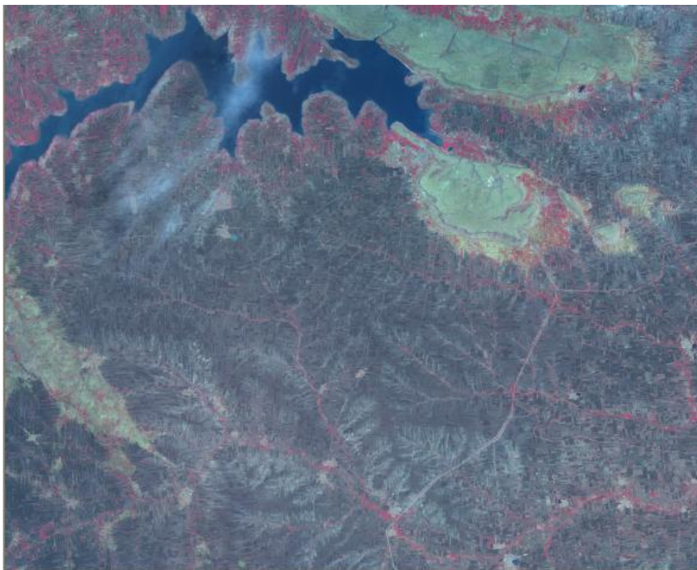
Fig. 9 (a) Standard FCC of the Landsat ETM+ image and (b) corresponding IHS transformed image
